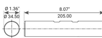
Technical drawing dimensions:  $\varnothing 1.36"$ ,  $\varnothing 34.50$ ,  $8.07"$ ,  $205.00$
