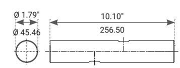
Technical drawing dimensions:  $\varnothing 1.79"$ ,  $\varnothing 45.46$ ,  $10.10"$ ,  $256.50$
